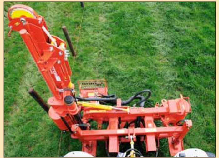
Aerial view showing rear shift and side shift operations in action. Note also the large flotation feet in contact with the ground. This gives brilliant stability on every type of terrain from rocky hill ground to very soft conditions.
