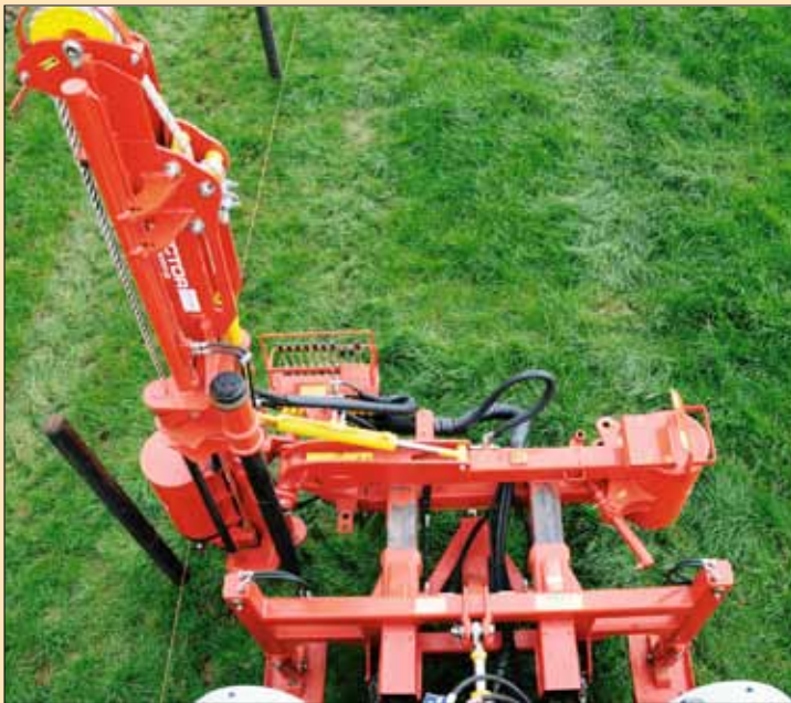
Aerial view showing rear shift and side shift operations in action. Note also the large flotation feet in contact with the ground. This gives brilliant stability on every type of terrain from rocky hill ground to very soft conditions.
