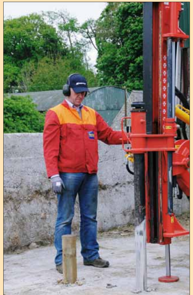
Rockspike Extractor in operation with hydraulic support jack under the mast.
