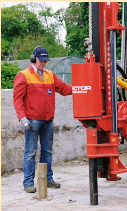
Vector Powerdrive Contractor demonstrating the unbelievable power of the rockspike attachment. Here the 90mm diameter hardened steel spike is being driven through 150mm of reinforced concrete.
