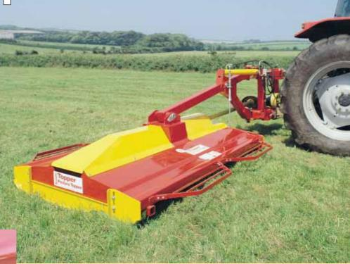
Pivoting Suspension system allows the Offset Topper to float over ground undulations. Spring cushioning is provided.
