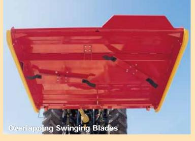
**The Hardened Spring Steel Blades** pivot on hardened bushes. The blades are cranked to reduce any possibility of stone damage. The tempered spring blade holders provide yet further protection against hidden objects.
