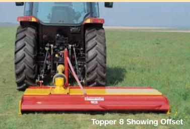
**Strong Simple Construction** incorporating high strength pressings result in a very robust machine. The smooth underside assists the flow of the cut material through the machine.
