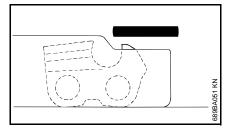
• Rework the depth gauge so that it is flush with the file gauge
