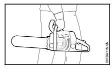
Always carry the chain saw by the handle – with the hot muffler away from your body, the guide bar must point to the rear. Avoid touching hot parts of the machine, especially the surface of the muffler – risk of burns!
