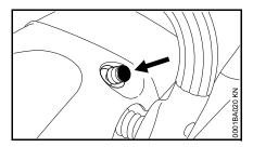
• Press in the button to open the decompression valve.
