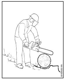
If on a slope, stand on the uphill side of the log. Watch out for rolling logs.
