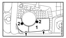
Insert cover plate (1) with both tabs (arrows) and fasten with the screws (2)
