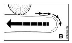
When the chain on the top of the bar – underbucking – is suddenly pinched, caught or encounters a foreign object in the wood, the chain saw may suddenly be driven straight back toward the operator – **to avoid this**:
