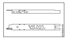
STIHL filing gauge (special accessory, see table "Sharpening tools") – a universal tool for checking sharpening and side plate angles, depth gauge setting, and tooth length, as well as cleaning grooves and oil inlet holes.
