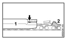
Lay the appropriate file gauge (1) for the chain pitch on the saw chain and press it against the cutter to be checked – if the depth gauge protrudes past the file gauge, the depth gauge must be reworked Saw chains with humped drive link (2) – upper part of the humped drive link (2) (with service mark) is lowered at the same time as the depth gauge of the cutter.
