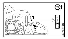
Press down trigger lockout and the blip the throttle trigger (2) – the Master Control lever (1) moves to the run position (I) and the engine settles down to idling speed.
