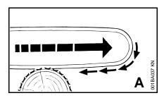
When the chain on the bottom of the bar – overbucking – is suddenly pinched, caught or encounters a foreign object in the wood, the chain saw may suddenly be drawn forward toward the log – to avoid this, engage the bumper spike firmly in the wood.
