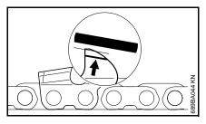
Afterwards, dress the leading edge of the depth gauge parallel to the service mark (see arrow) – when doing this, be careful not to further lower the highest point of the depth gauge
