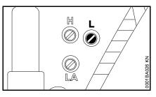
Determine the required standard setting as follows: Turn the low speed screw (L) carefully clockwise as far as stop, then turn it counterclockwise.
