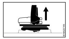
• Remove the tank cap.
