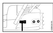
• Unscrew the nuts and take off the chain sprocket cover.
