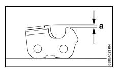
The depth gauge determines the depth to which the cutter penetrates the wood and thus the chip thickness.
