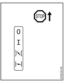
$\begin{array}{l} \textbf{Stop 0} - \textbf{engine off} - \textbf{the ignition is} \\ \textbf{switched off} \end{array}$
