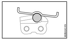
• Guide the file: **horizontally** (at a right angle to the side surface of the guide bar) in accordance with the specified angle – according to the
