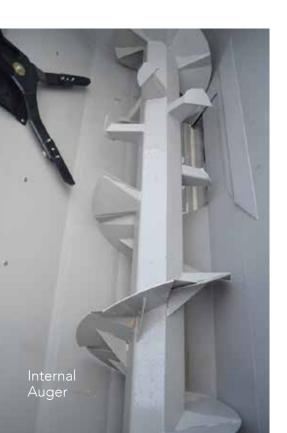
The Powerspread principal uses a full length 33" diameter welded steel auger turning at 13 rpm, this moves material from both the front and rear of the hopper towards the centrally mounted door. The door opens vertically so that 100% of the width of the discharge rotor is utilised at all times.
