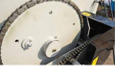
New uprated chain drive system with 16mm shearbolt
