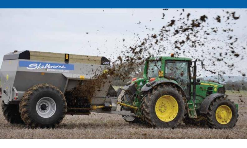
THE POWERSPREAD DAIRY RANGE IS DESIGNED AS A STRONG SIMPLE MACHINE FOR SPREADING A WIDE RANGE OF SOLID AND LIQUID FARMYARD MANURES AND WASTES.
