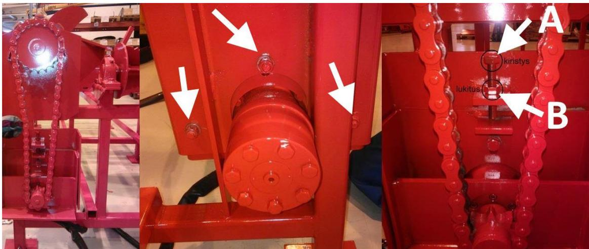
*Figure 5 (tightening the motor chain)*
