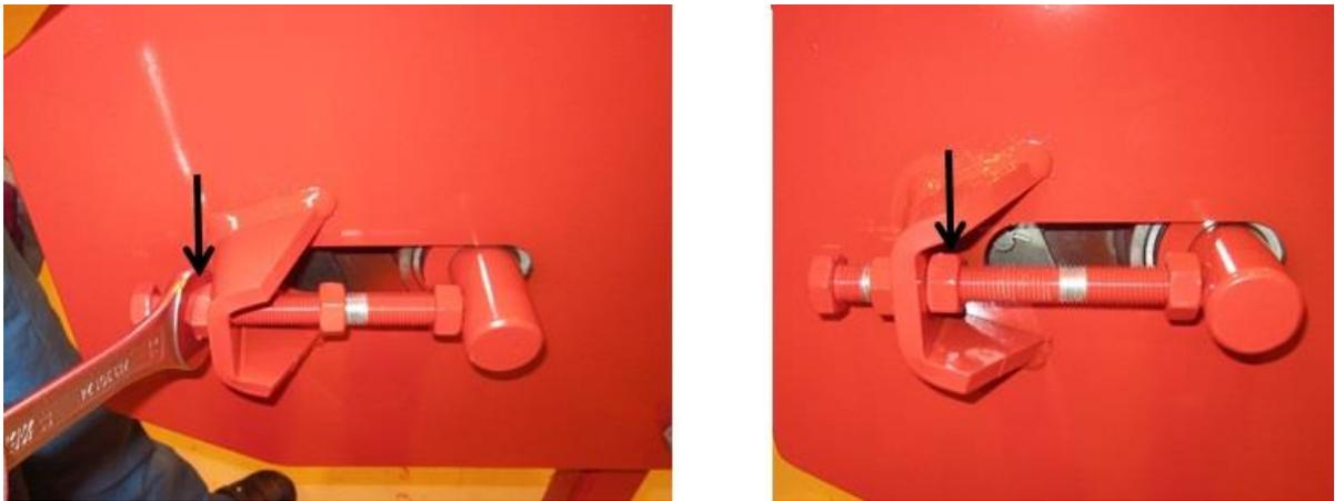
Figure 4 (Adjusting the tightness of the chain conveyor's chains)
