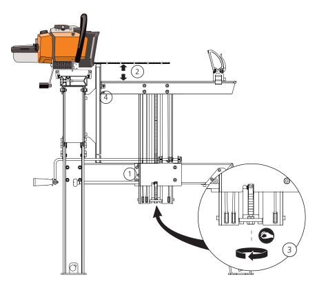
Check that when the log lifter is cranked down, it moves easily through the ratchet cam housing driven by its own weight.
