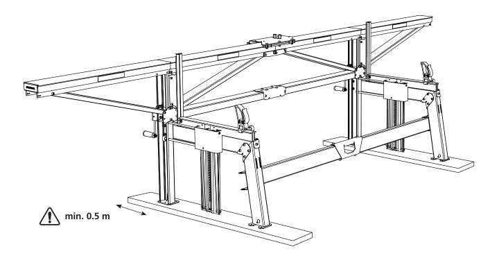
When the sawmill is placed directly on the ground, the surface must be firm and level enough to drive a regular passenger car on.
