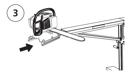
Push the carriage onto the guide rail with the guide bar in the direction of the log beds.
