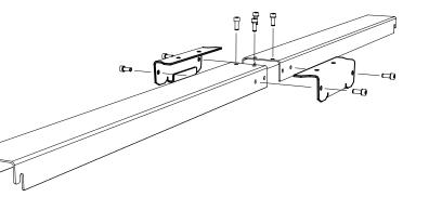
Fit the guide rail struts to both sides
