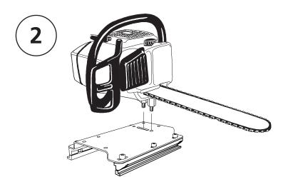
Fit the Logosol nuts through the track in the carriage. Tighten the chainsaw into place by using the chainsaw's guide bar nuts under the plate.
