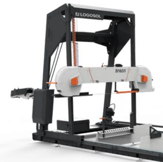
The light metal band wheels are combined fan wheels that cool the saw blade and act as an air brake. The fan wheels blow away the sawdust and keep the inside of the saw head and the workplace clean and tidy. This is a great advantage when changing blades and servicing.
