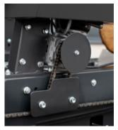
**Extra-reinforced log bed that can be easily extended** The B1651 has reinforced log shelves, reinforced rail construction, extra feet under the log shelves and reinforced, torsional rigid saw bed ends.
