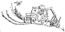
Minimi: tractor and trailer tilt, the more the weight is displaced to the point where they can turn over.
