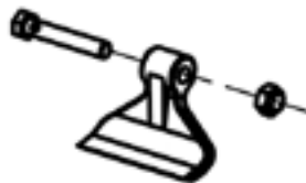
Installation of hammer flail
