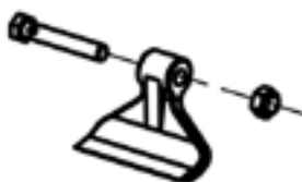
Installation of hammer flail
