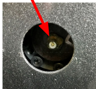
Lubricate the coupling , otherwise the bearing will cut and the coupling will break.
