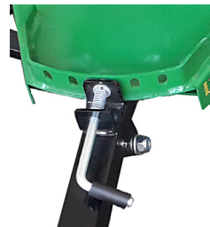
Lever. Lateral adjustment of tow bar
