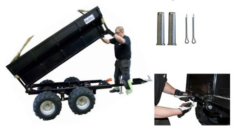
• The hydraulic cylinder must be fitted while the floor is raised. **WARNING!** It is important that you ensure that the floor cannot drop down! Connect electric cables to a 12V battery in order to start the hydraulics. Extend the cylinder so that the piston rod reaches the bracket under the floor, secure with the pin.
