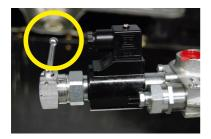
Emergency use of electric valve without using the levers. When the vehicle has not been in use for a longer while, the radio control can start to feel harsh or stop working. The electric valve is equiped with mechanical levers on each side that can be used in emergency situations.
