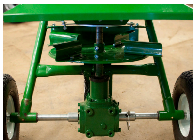
Spreading plate with 4 spreader blades.
