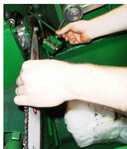
3. Install a new chainsaw bar / chain, then fit the bolts. Do not tighten the bolts completely until the chain is properly tensioned
