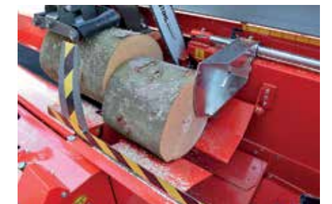
The guide plates ensure that even the shortest pieces of wood fall neatly into the splitting groove.
