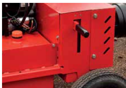
Power transmission can be released and engaged with a lever.
