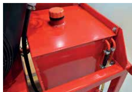
Large 32 l fuel tank enables uninterrupted use of the firewood processor. Fuel level can be checked from a display.
