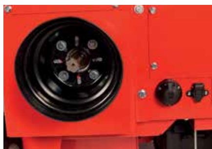
Protected PTO and power supply connections.
