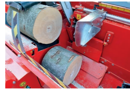
The log landing plates ensure that even the shortest cut logs land neatly into the splitting groove.
