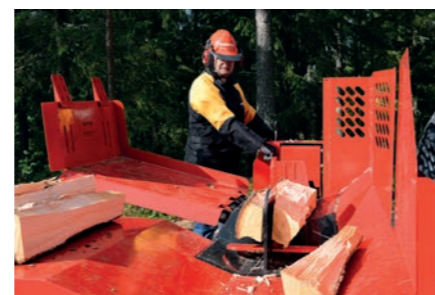
Thanks to the hydraulic height adjustment, you can split the log into two or four pieces by adjusting the height of the splitting blade.
