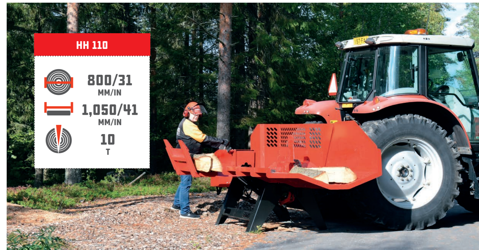
Thanks to the hydraulic height adjustment, you can split the log into two or four pieces by adjusting the height of the splitting blade.
