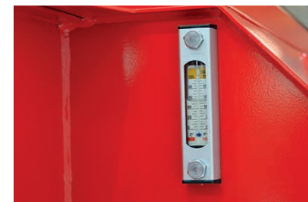
Large oil tank capacity and sight glass.
