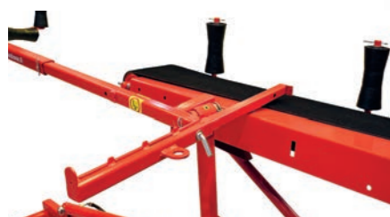
The transport support is pulled out from the arm and over the infeed conveyor.
