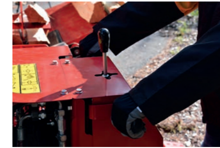
Easy to operate with lever control in which splitting is done with two hands.
