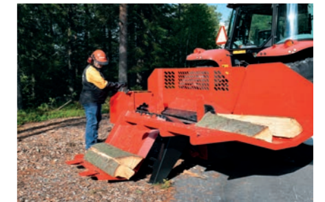
The hydraulic log lifter allows large logs to be handled without strain.
