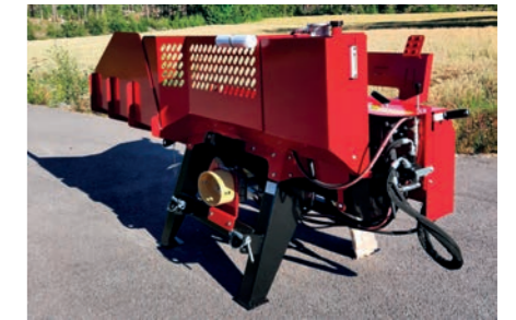
Hakki Pilke HH 110 OH has its own hydraulics with a recommended output of 400 r/min, 37 l/min.
