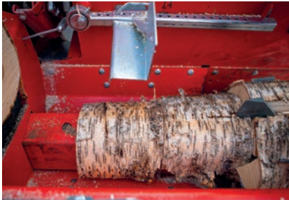
38 Pro has a halfstroke function for making the splitting process of short firewood faster. The half-stroke splitting can be easily controlled with a button in the front panel.
