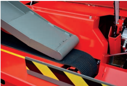
Log feed using a heavy duty belt with a rough surface.
