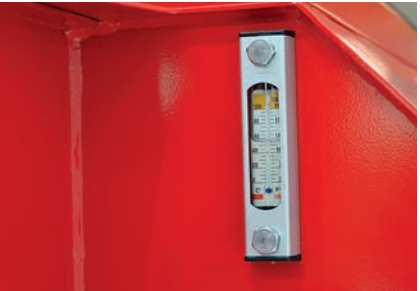
Large oil tank capacity and sight glass.
