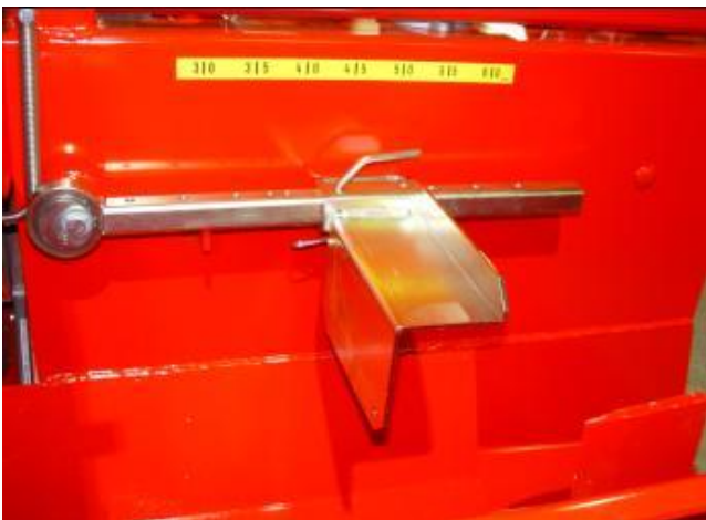
Figure 26. Limiter plate position for small logs.
