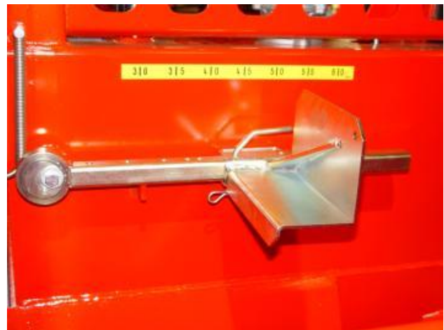
Figure 27. Limiter plate position for large logs (diameter over 20 cm).
