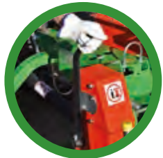
Emergency braking device for models with PTO
