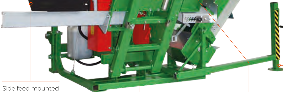
Lever for unlocking the bench movement (Exclusive THOR system)
