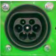
Standard Type 2 charging inlet on loader
