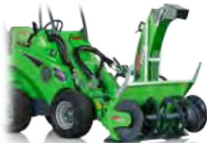
Option: Electric throwing height adjustment A430172
