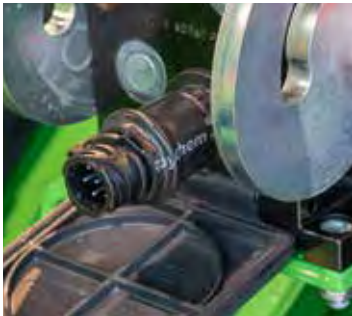
Adapter cable for attachment's multi connector A36679
