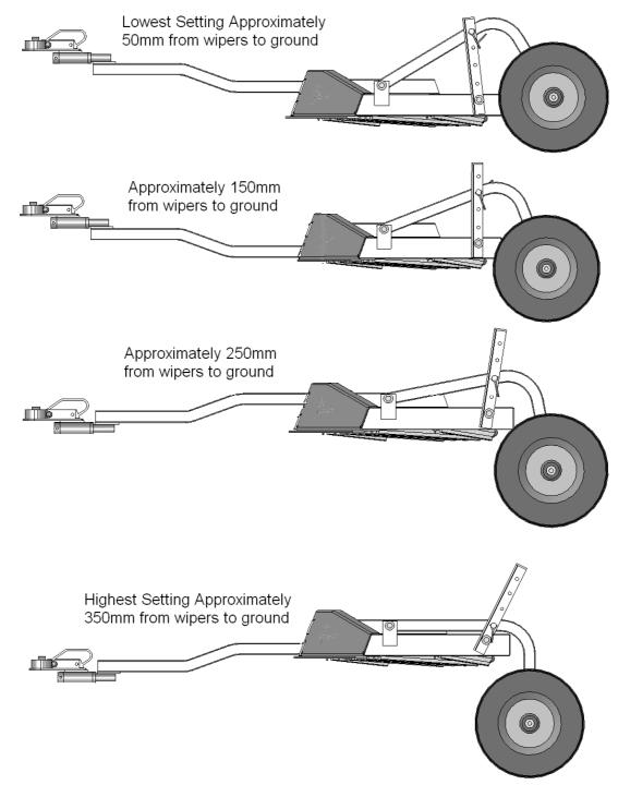
On the Winged Eliminator unit the wings has adjustable skids to match up the height of wings to centre frame to give consistent wiping height.
