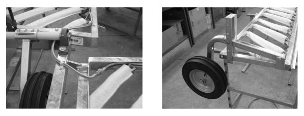
Fit the wings to the main frame – use washers as spacers on the shoulder bolts if required. Fit the RH & LH axles and height adjusters. Fit wheels to all the axles.
