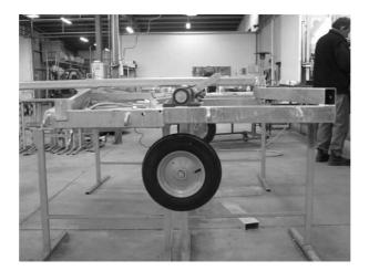
Lower the suspension and fit the wheels
