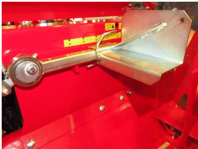
Figure 20. Limiter plate position for large logs of more than 25 cm in diameter
