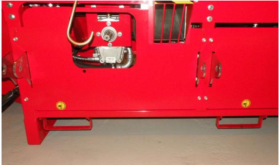
Figure 12. Lifting points of the machine
