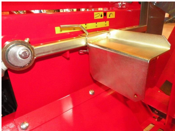
Figure 19. Limiter plate position for smaller logs
