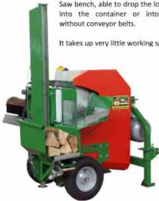
Saw bench, able to drop the logs off directly into the container or into the trailer, without conveyor belts.
