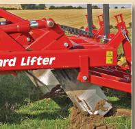
Leg protection is provided by either shear-bolts or a hydraulic auto-reset system to prevent damage from large obstacles under
