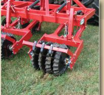
Individual spring loaded heavy cast Prisma press rollers follow immediately behind each leg to close and level the surface leaving your field ready
