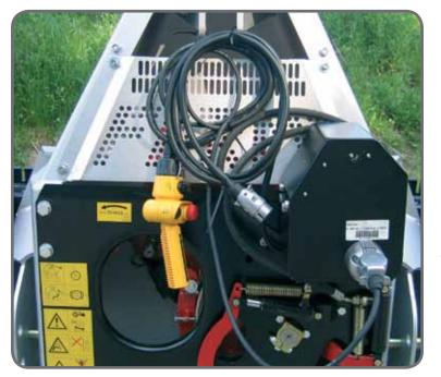
Instead of the electric control system, a radio control system can be installed at the same position.
