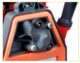
Filter support with carburettor anti-backflow element (Emak patent): prevents the filter from becoming fouled by fuel and guarantees longer operation between filter maintenance operations.
