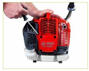
"Easy on" device: composed of a double spring in the starter cover combined with driver with two ratchets means reduced force with each pull and fast starting with fewer rope pulls.
