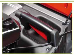
The centralized cutting height adjustment device controlled by a rugged and ergonomic handle provides 5 different height positions that can be selected easily and effortlessly from a minimum of 28 mm to a maximum of 75 mm.
