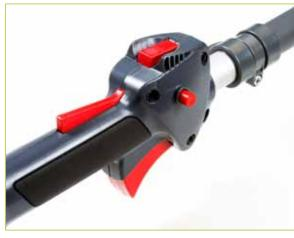
On/off switch: returns automatically to the "on" position after each stop (always on).
