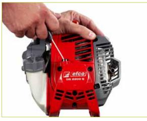
"Easy on" device: composed of a double spring in the starter cover combined with driver with two ratchets, this device means reduced force with each pull and fast starting with fewer rope pulls.
