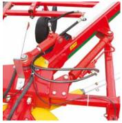
Hydraulic working width adjustment
