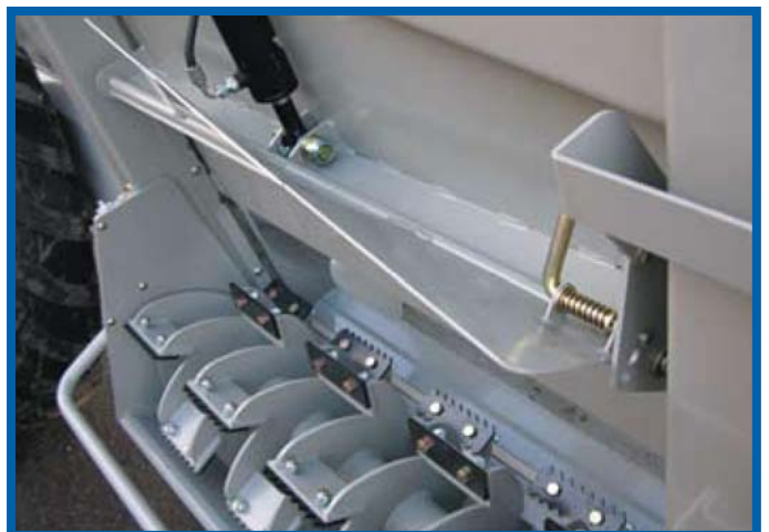
Adjustable slurry deflector controls discharge height
