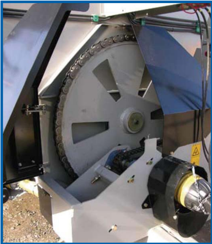
Simple high power chain drive with reverse
