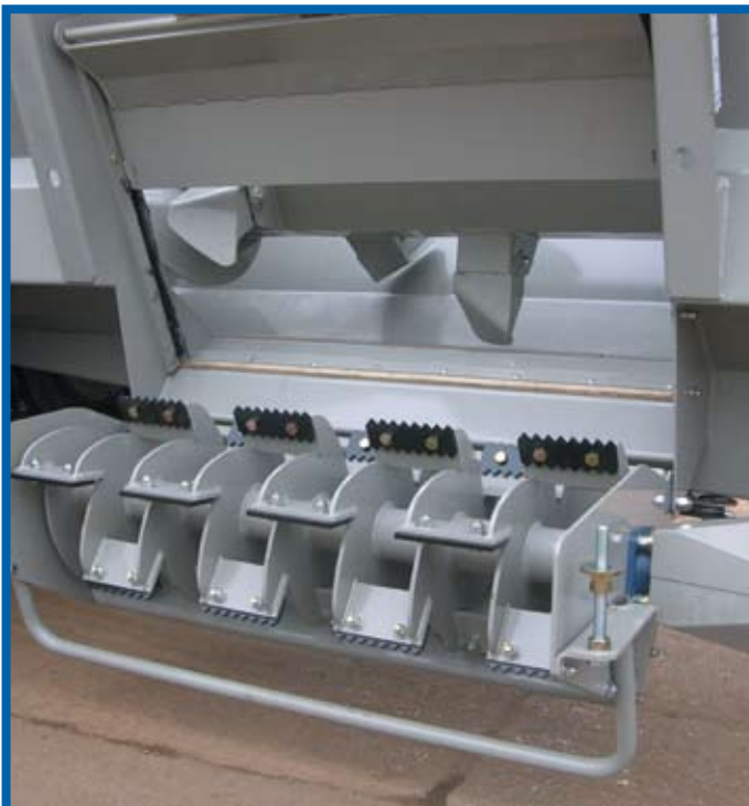
Discharge rotor can be hydraulically lowered to allow access
