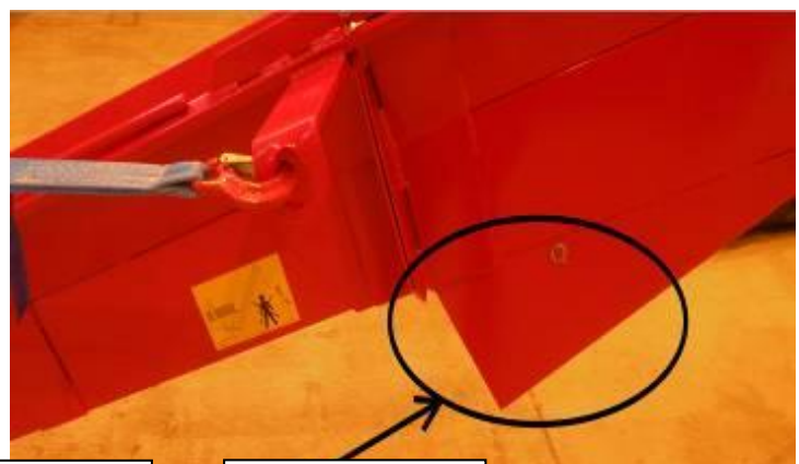
Belt tightness adjustment screw C (2 pcs/conveyor)
