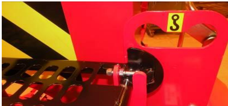
Figure 4. Lifting points for a chain or strap.
