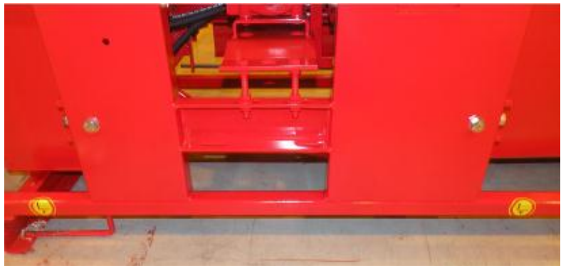
Figure 3. Lifting points for a forklift.
