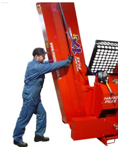
3. Pull the conveyor until the line of the winch tightens
