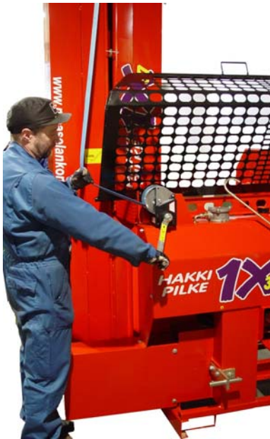
1. Unwind some line from the winch
