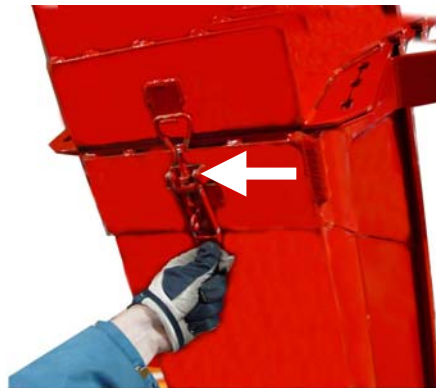
7. Adjust the conveyor with the winch to desired inclination and lock it with the lock in the bottom of the conveyor and ring cotter.
