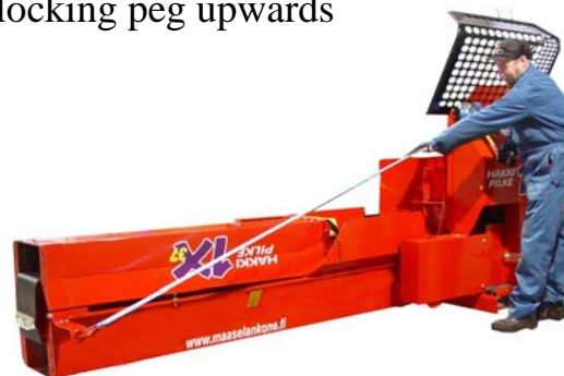
4. Lower the conveyor with the winch to horizontal position
