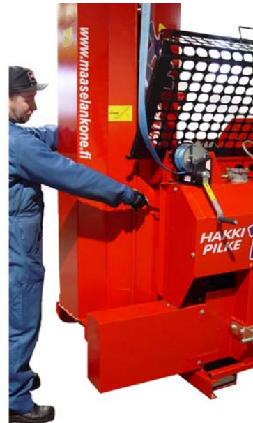
2. Push the conveyor towards the machine and release the locking of the conveyor by lifting the locking peg upwards
