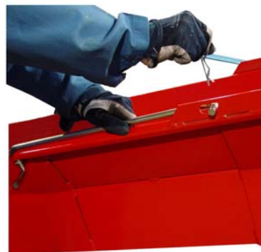
8. Swing the belt holder to the side of the conveyor
