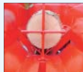
With the standard blade the wood can be split into 2 or 4 pieces. A blade that splits into 6 pieces is also an option.
