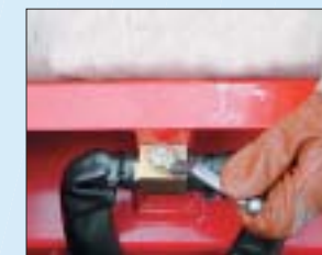
The acceleration valve allows a fast cycle time (33% faster) for small diameter logs and full splitting force for large diameter logs (optional extra).
