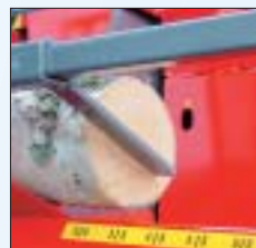
Log length can be measured quickly and easily and pre-set to the desired length. The log stop deflects as the log is cut, allowing the wood to fall unobstructed into the splitting chute.
