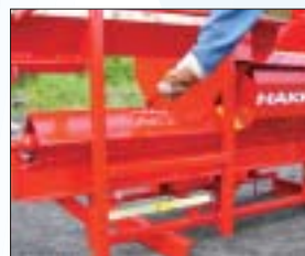
If necessary, the operator can stop and reverse the splitting cycle.
