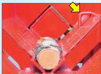
As the log drops into the splitting chute it activates the splitting mechanism.
