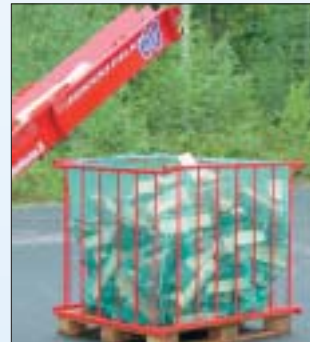
Net sack support frame for bagging the firewood directly from the conveyor.
