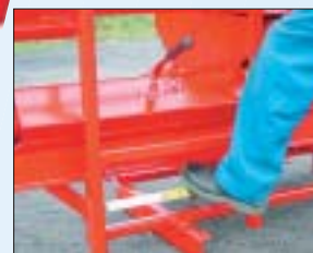
Triggering the splitting movement by foot.
