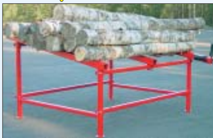
Log rack can be loaded with a grapple and allows easy transfer of the logs on the machine.
