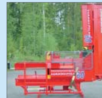
When not in use, the conveyor is folded and locked in the vertical position.
