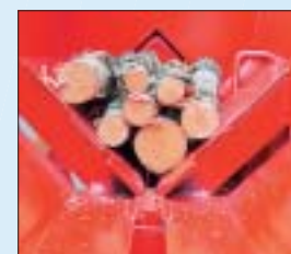
The 'V' shaped chute ensures logs are always positioned central to the splitting blade.
