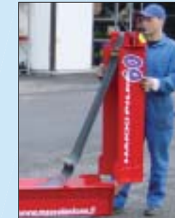
The conveyor folds easily for transport.
