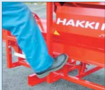
In an emergency, all the functions of the machine are stopped using a foot operated pedal.
