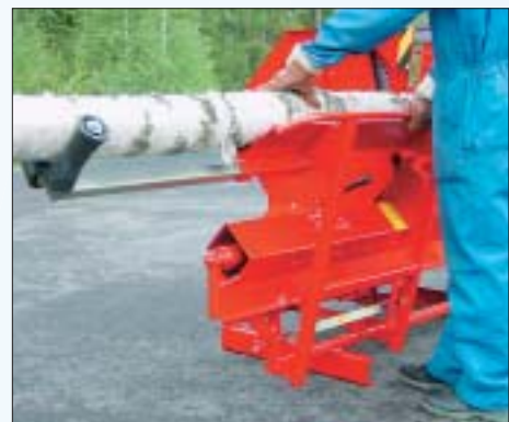
Ergonomically correct, balanced crosscut table is fitted with contoured log support rollers.
