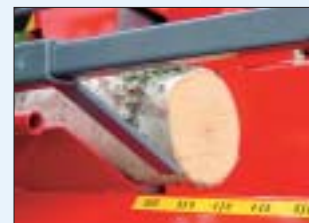
Log length can be measured quickly and easily and pre-set to the desired length. The log stop deflects as the log is cut, allowing the wood to fall unobstructed into the splitting chute.
