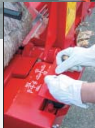
All functions of the machine are operated hydraulically: log feed, cross-cutting and height adjustment of the splitting blade.
