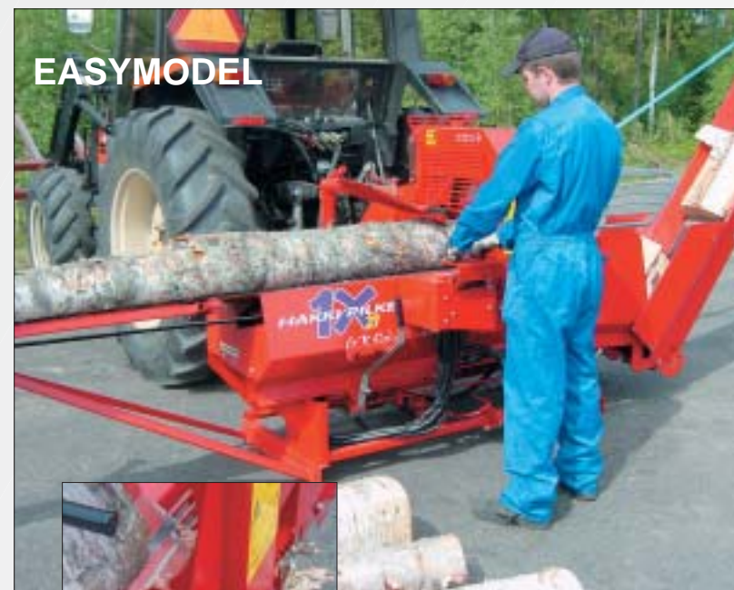
The feed conveyor carries the log into the machine. Machine operation is by the hand lever.
