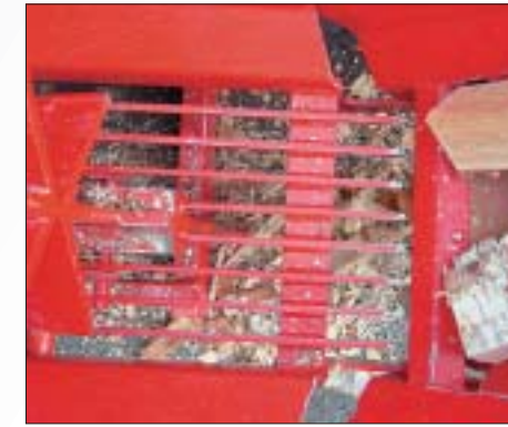
After splitting the firewood passes over a grid through which wood waste and splinters can fall.
