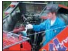
The conveyor height is adjusted with a hand operated self-locking winch.
