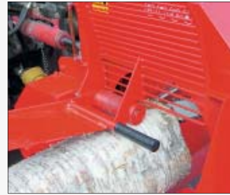
The spring-loaded support roller automatically opens the guard.
