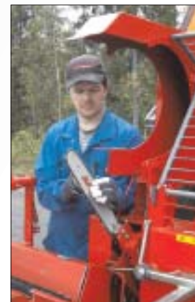
The sawbar cover is opened using a spanner. This allows easy access for maintenance.
