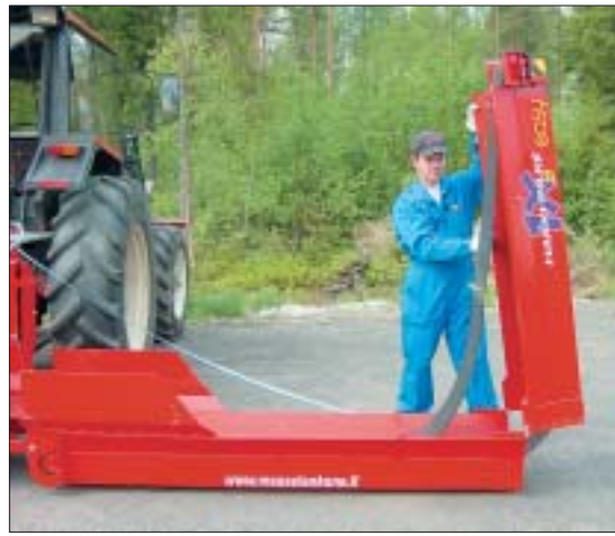
The 4 m conveyor folds easily for transport.
