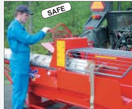
Ergonomically correct working position: cutting with the right hand. Cutting and splitting takes place in a fully guarded area.
