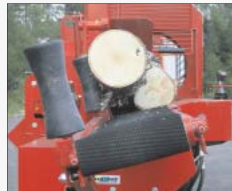
The slightly inclined infeed conveyor keeps twisted wood on the table.
