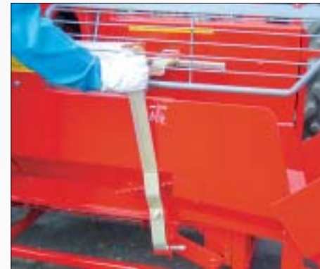
Blade height adjustment is quick and easy.
