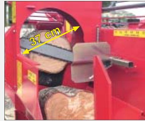
Maximum log diameter 37 cm. Splitting force 5,5 T. A 7, 0 T splitting cylinder is optional.
