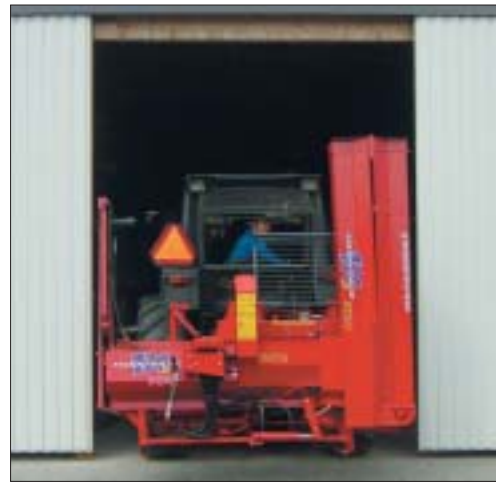
With the conveyors folded the machine is compact for transport and storage.
