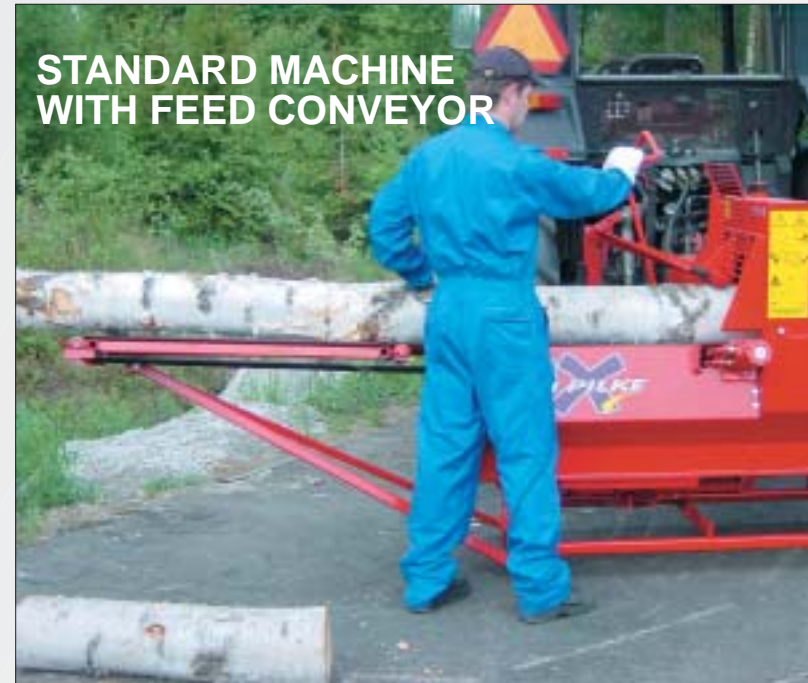
The feed conveyor carries the log into the machine. Machine operation is by the hand lever.
